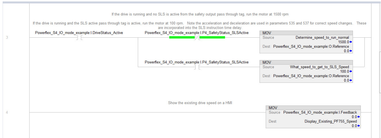
Figure 61 – Standard I/O Routine That Runs the Drive at Velocity and Changes to Safe Limited Speed Velocity When Requested by the Safety Task
